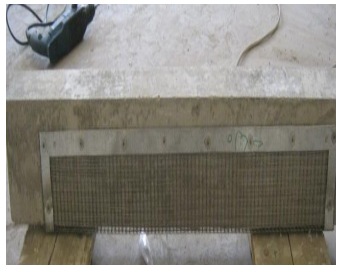
Figure 1 steel wire mesh and transverse steel straps.
