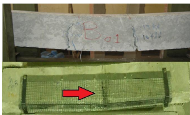
Figure 6 beams after failure and strengthened under the existing deformation
