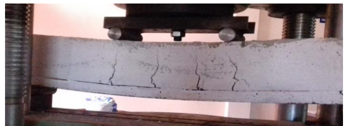
Fig. 8: Bending Failure of Strengthened Beam
