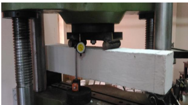
Fig. 4: Testing Setup for Control Beams
