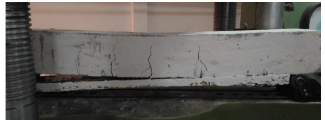
Fig. 7: Combined Bending & De-bonding Failure
