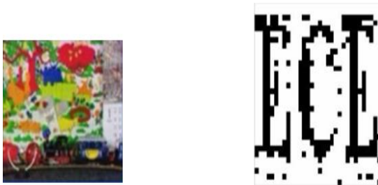
Fig 1.9. Low pass filtered watermarked mobile video frame and Retrieved watermark with BER=0.06543
