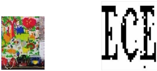
Fig 1.7 Resized (144x144) watermarked mobile video frame and Retrieved watermark with BER=0.017578
