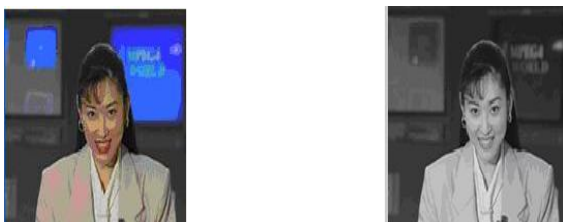
Fig 1.11. a) Watermarked akiyo video frame and its Luminance Channel with average MSE=14.4441, average PSNR=36.9378 dB and Embedding time = 22.2464 sec
