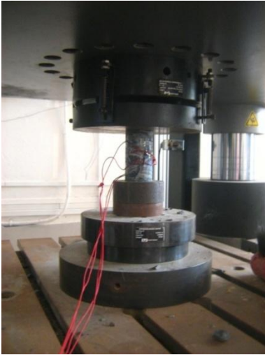
Fig 3.3 Experimental setup for UCS testing
