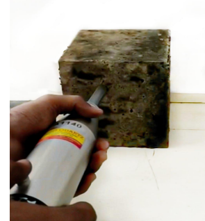
Fig. 2. Rebound hammer test
