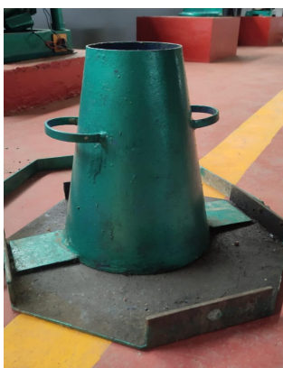
Fig. 1. Slump cone test
