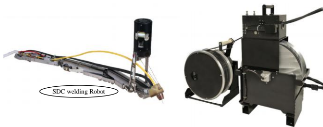
Figure 10. Diakont welding robot and deployment station with welding rod pusher [5]
