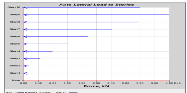
Fig 7- Storey Lateral Loads for Model 2(Infill Frame)
