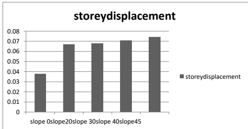
Fig.8. Bar graph showing story displacement in X-direction at different slopes
