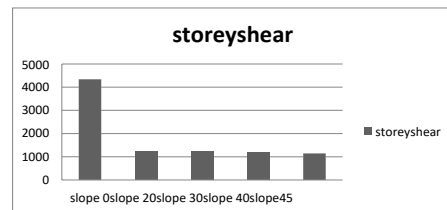
Fig.7. Bar graph showing storey shear in X-direction at different slopes
