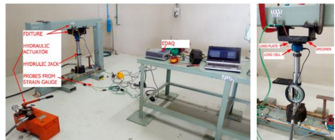
Fig. 8. Fixture and experimental set up
