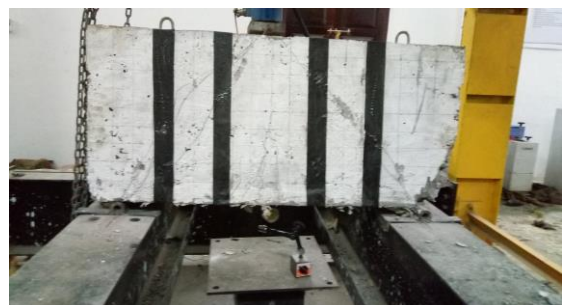
Fig 6. Retrofitted beam after failure
