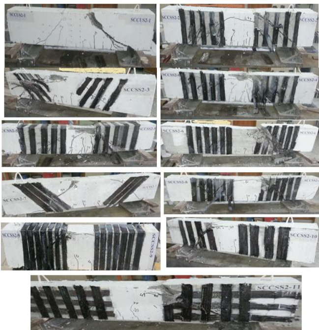
Figure(4): Pattern cracks
