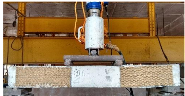
Fig. 4. Testing of the beam under four point loading.
