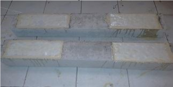
Fig. 2. Beams retrofitted using epoxy binder and glass fiber.
