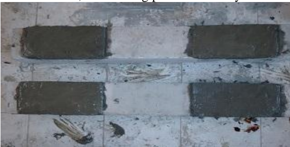
Fig. 3. Beams retrofitted using cement matrix composite and sisal fiber.
