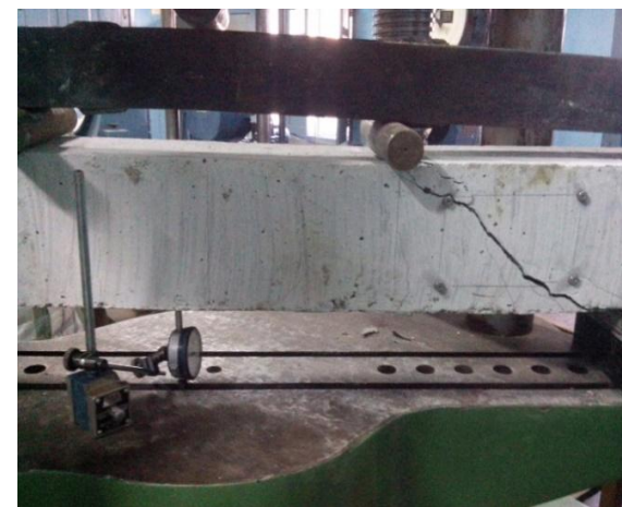
Figure 4.3 Crack pattern of the Beam
