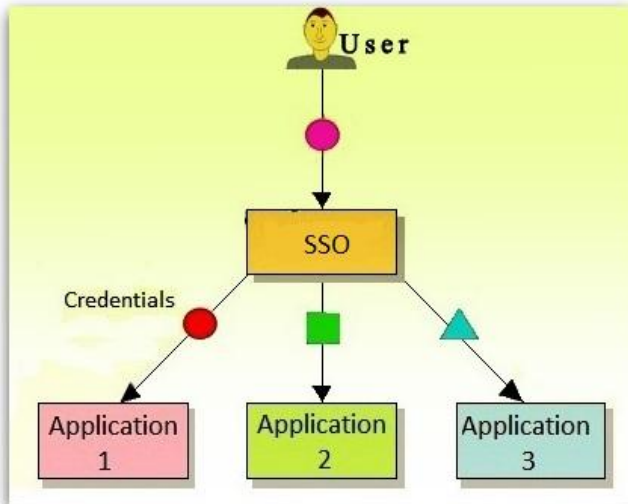
Fig. 2. Single logon procedure for a user employing an SSO Tool, where credentials come from the SSO tool
