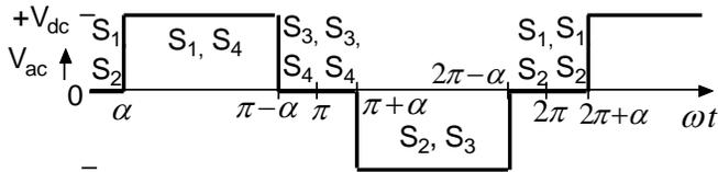
Fig. 2. AC output voltage of a single H-bridge.
