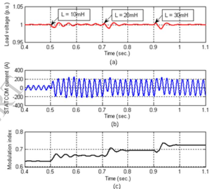
Fig. 12. Effect of varying coupling inductor on (a) ac system dynamic response, (b) dynamic response of the STATCOM output current and (c) variation of modulation index.
