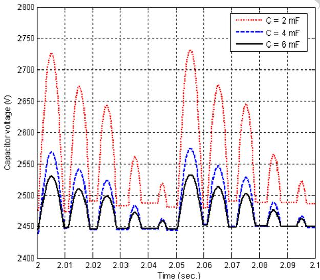
Fig. 5. Voltage ripples for different values of dc capacitance for  $v_{dc} = 2500$  V for  $m = 0.8$ .
