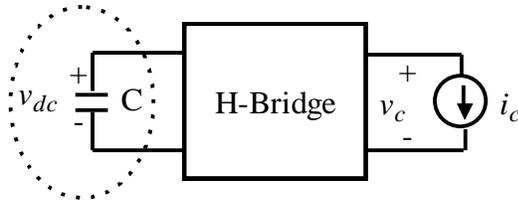
Fig. 4. DC capacitor utilized in an H-bridge of CMLI.
