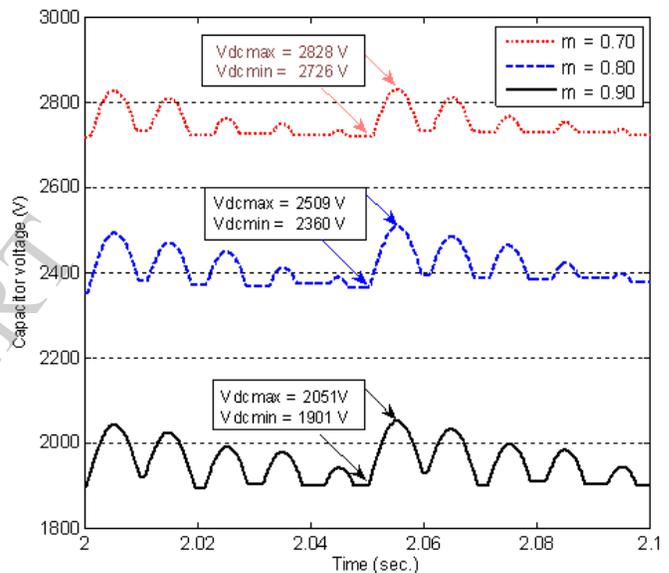
Fig. 6. DC voltage ripples across capacitor for different values of modulation indices at  $C = 4$  mF.
