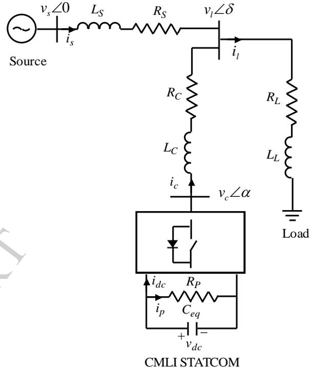
Fig. 3. Single-line diagram of CMLI based STATCOM.
