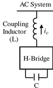
Fig. 10. Coupling inductor used in STATCOM applications.
