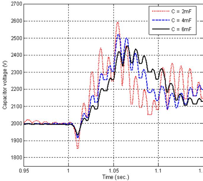
Fig. 7. DC voltage across the capacitors under a step change in the STATCOM output current.
