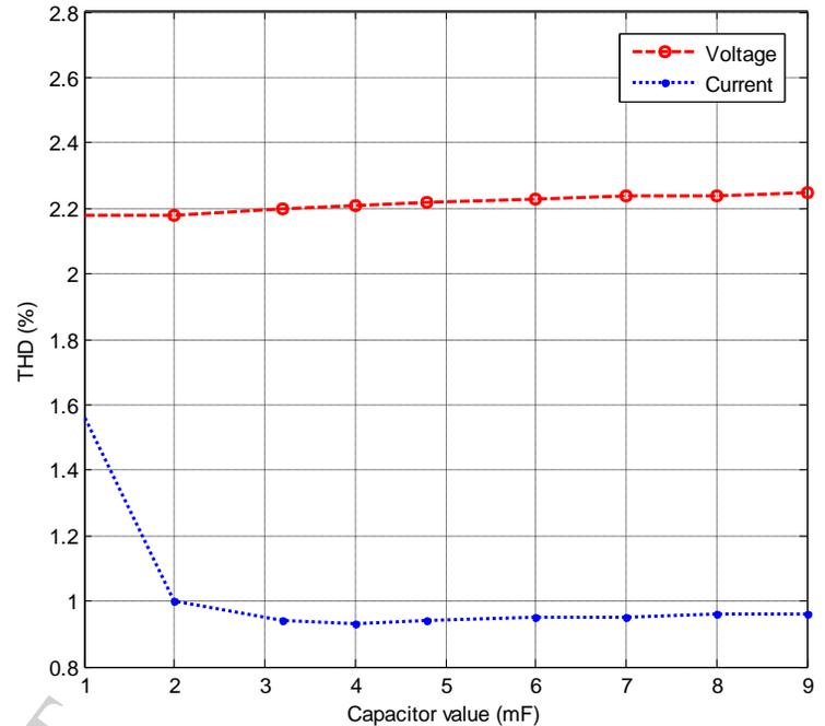
Fig. 9. The variations of harmonic distortion in the output voltage and current of the STATCOM as a function of DC capacitor at  $m = 0.9240$ .
