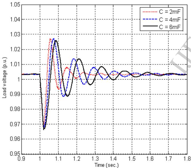
Fig. 8. Load voltage variations when a step load change occurs.
