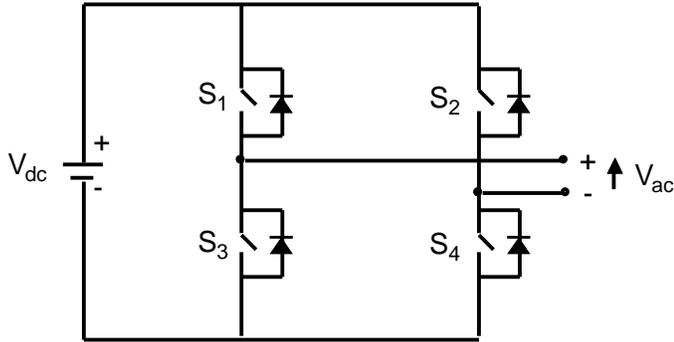
Fig. 1. An H-bridge of cascade multilevel inverter.
