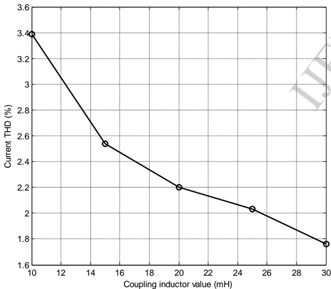
Fig. 11. Variation of the STATCOM output current THD as a function of coupling inductor.
