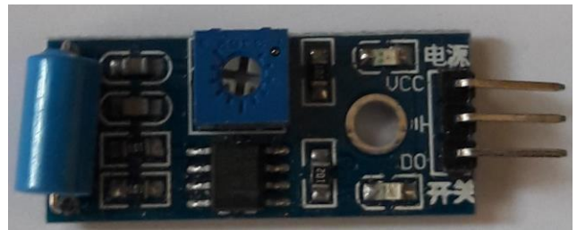
Fig6: Piezo vibration sensor detects mechanical vibrations
