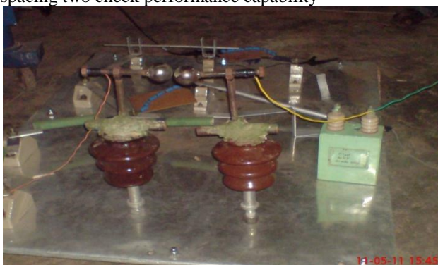
Figure 6. Completely designed impulse voltage generator
