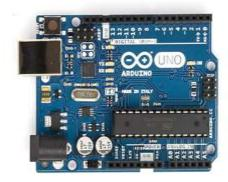
"Uno" means one in Italian and was chosen to mark the release of Arduino Software (IDE) 1.0. The Uno board and version 1.0 of Arduino Software (IDE) were the reference versions of Arduino, now evolved to newer releases. The Uno board is the first in a series of USB Arduino boards, and the reference model for the Arduino platform; for an extensive list of current, past or outdated boards see the Arduino index of boards
