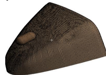
Figure 6-FE model of cowling structure
