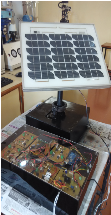
Figure 10. Integrated solar smart inverter system
