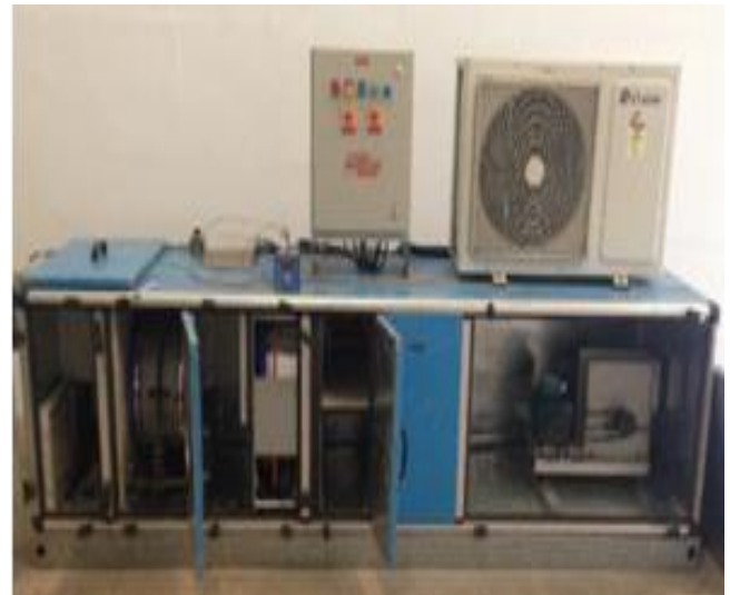
Figure: 1. Photographic View of Solid Desiccant assisted Hybrid Air-Conditioning System setup
