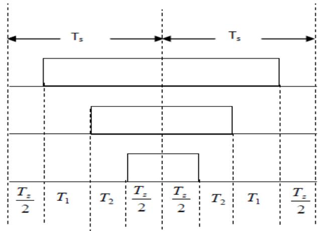
Figure 2(a): Sequence and gating times in sector 1 for proposed SVPWM
