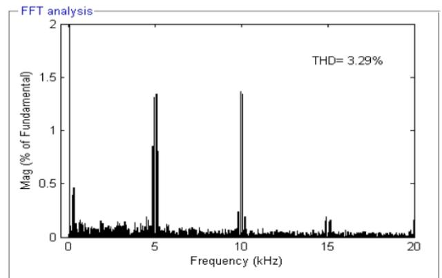
Figure 9: Harmonic spectra for line currents for conventional direct torque controlled induction motor drive
