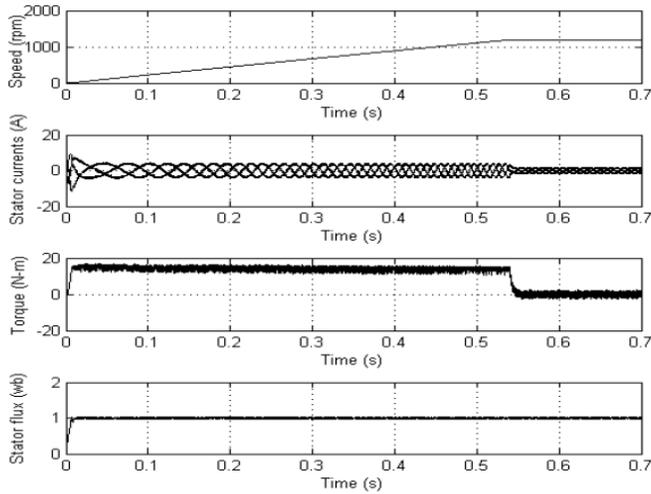
Figure 4: Starting transients and steady state plots for conventional direct torque controlled induction motor drive
