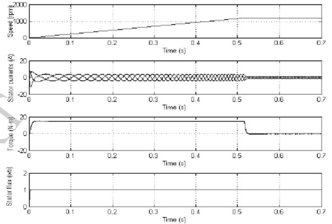
Figure 8: Starting transients and steady state plots for conventional SVPWM direct torque controlled induction motor drive
