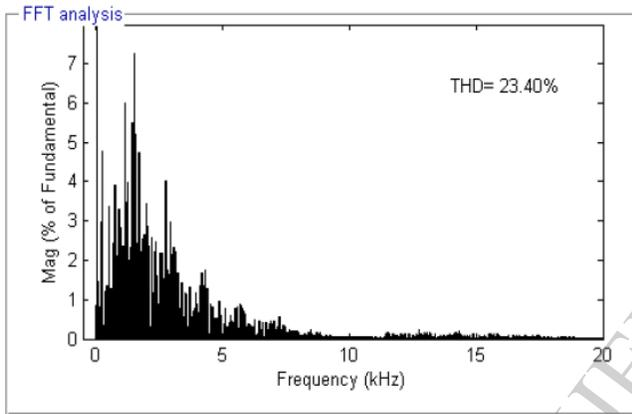
Figure 5: Harmonic spectra for line currents for conventional direct torque controlled induction motor drive
