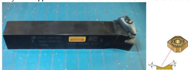
Fig. 2. Turning tool holder and cutting tip used
