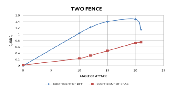
Graph3: C_L AND C_D for airfoil with two fences
