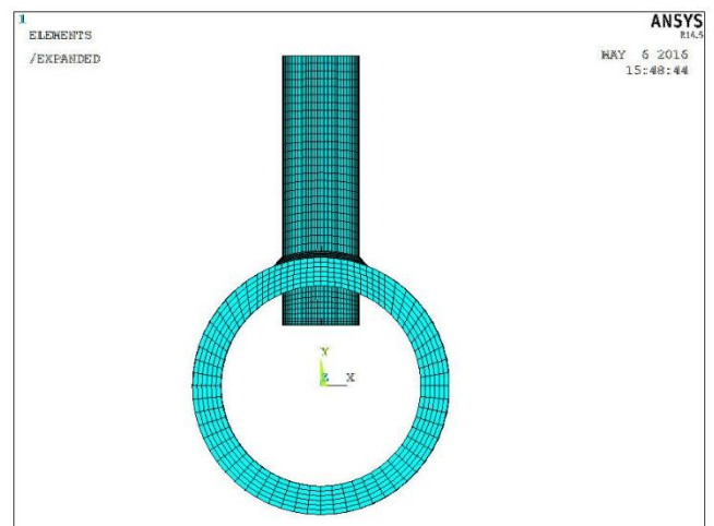
Fig 13: ANSYS model of partial penetration weld joint
