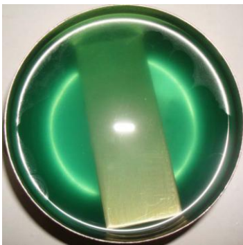
Figure 4.2.2. Brass plate immersed in SA after 200 thermal cycles
