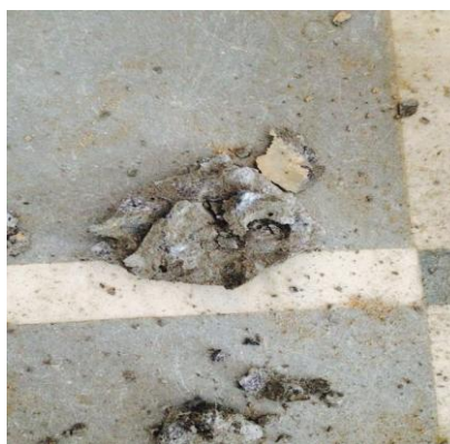
Fig 6. Cube with 100 % of steel slag after testing
