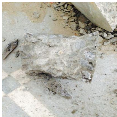
Fig 5. Cube with 0 % of steel slag after testing
