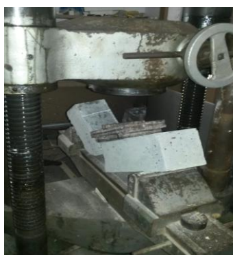
Fig 8. Flexural strength test for beam
