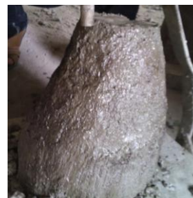
Fig 2. Slump test at 0% of Steel slag
