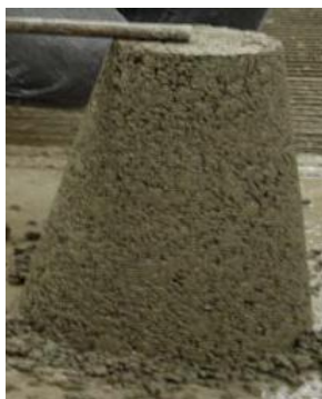
Fig 3. Slump test at 100% of Steel slag
