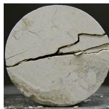
Fig 10. Split Tensile strength for cylinder
