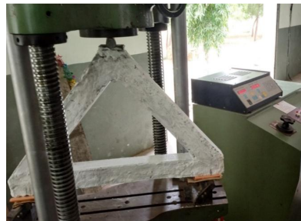
Fig 6 Test setup of Concrete Infill Specimen
