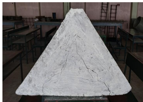
Fig 10 Failure crack pattern of STM 3C
