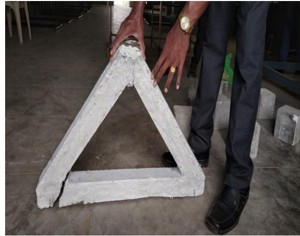
Fig 8 Failure crack pattern of STM 1
