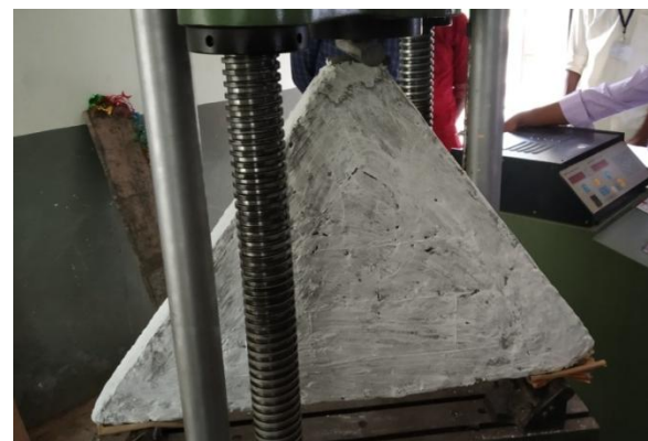
Fig 7 Test setup of Masonry Infill Specimen
