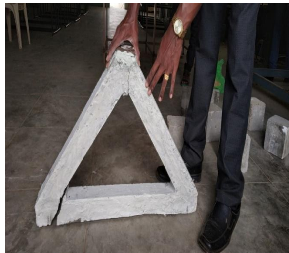
Fig 11 Experimental failure profile of STM 1
