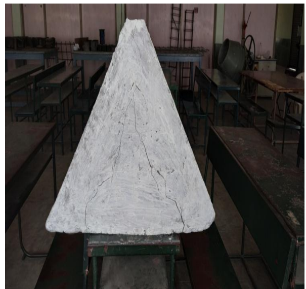
Fig 15 Experimental Failure profile of STM 3C
