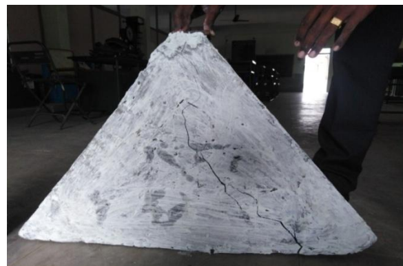
Fig 9 Failure crack pattern of STM 2M
