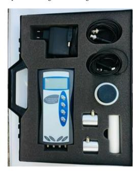
**Transducers:** These are the sensors that transmit and receive the ultrasonic pulses. They are typically attached to the surface of the building material being assessed. Make sure you have transducers suitable for the type of material you are testing.
