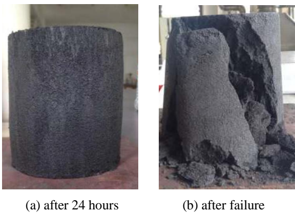
Fig. 2 Prepared sample before and after unconfined compression test.
