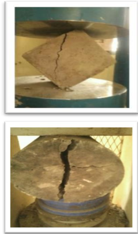
Figure 4 Tensile Test set up
