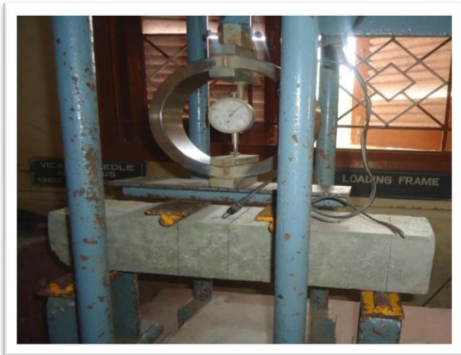
Figure 3 Flexure Test set up
