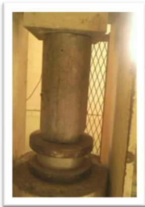
Figure 1 Compressive test set up
