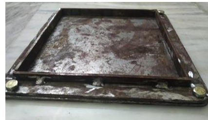
Figure 1: Mould of size 150mm x 150mm x 10 mm prepared for casting of geopolymer concrete tile specimens
