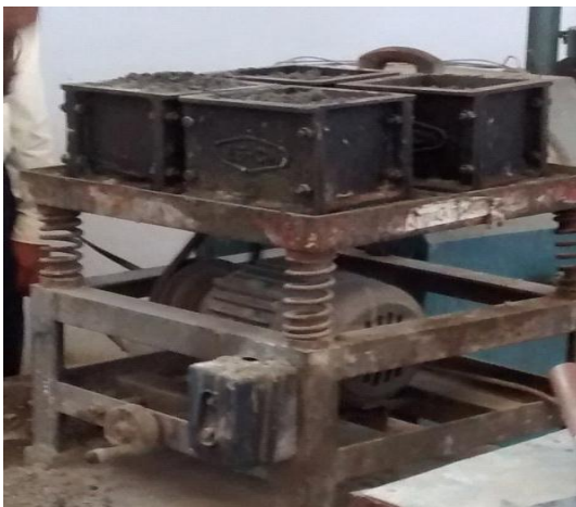
Fig1 Casting of cubes
