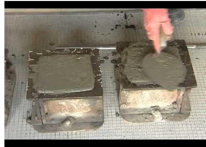
Preparation sample of nano concrete blocks
