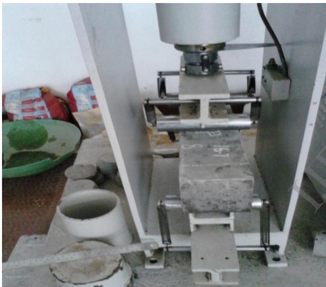
Fig. 4 Reinforced beam placed for flexural testing
