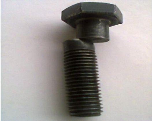
Figure 15 Bolt Sheared along shank region
