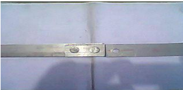
Fig. 7 Failure of test specimen
