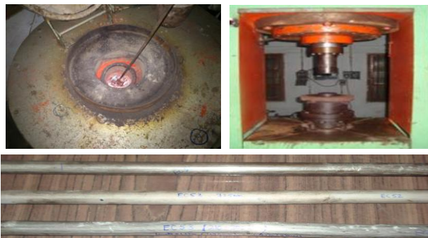
Fig. 1 Production of composites by stir casting and Extrusion
