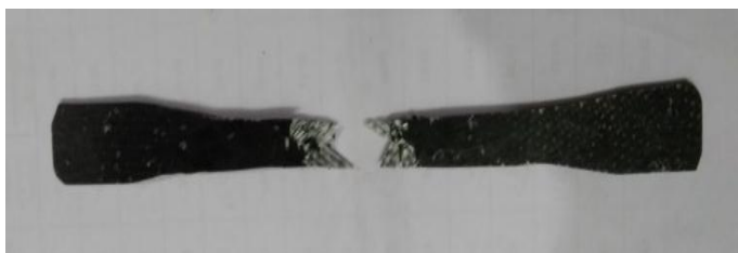
Fig 8.1: Fractured specimen after tensile testing of 30° orientation.
