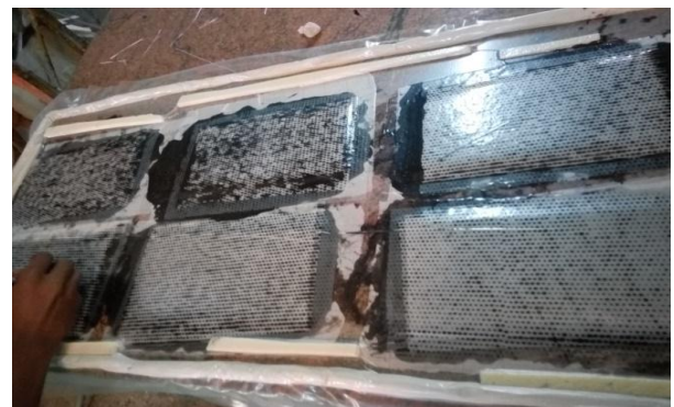
Fig 4: GFRP Laminate Fabrication by Vacuum Bagging Technique
