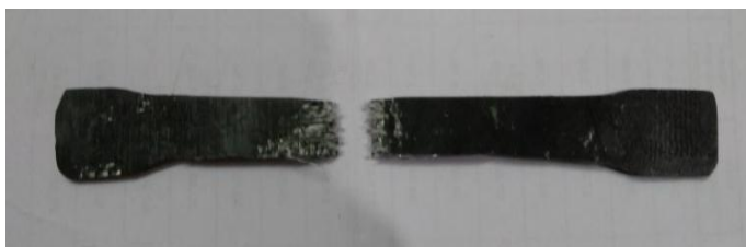
Fig 8.3: Fractured specimen after tensile testing of 90° orientation.
