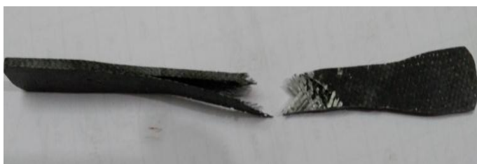
Fig 8.2: Fractured specimen after tensile testing of 60° orientation.
