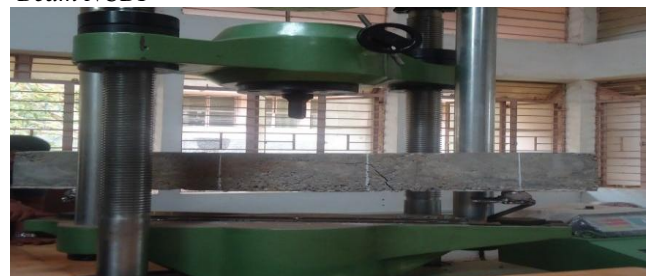
Figure7: Failure of beam NCB1
