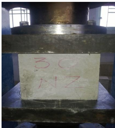
Fig 4: Compressive Strength Test
