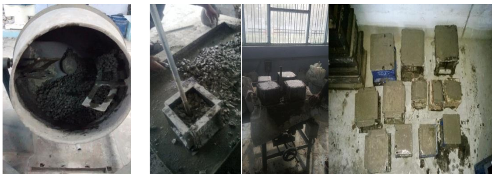
(b) Machine Mixing(c) Compaction of Specimens(d)Casted specimens
