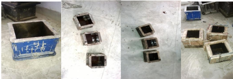
(a) Different sizes of cube moulds used in the project (viz: 150mm, 125mm, 100mm, 75mm)
