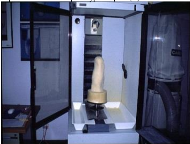
Fig.3 Prototype prosthesis using FDM
