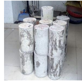
Figure 1 Wrapped concrete specimens
