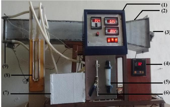
Figure 1: Experimental Equipment: (1) Display, (2) Air flow duct, (3) Forced draft fan, (4) PID controller, (5) Rotameter, (6) By pass valve, (7) Reservoir tank, (8) U tube manometer, (9) Heat exchanger.
