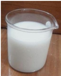
Figure 4: 0.1% volume concentration Al<sub>2</sub>O<sub>3</sub>/water and ethylene glycol (60:40) nanofluid
