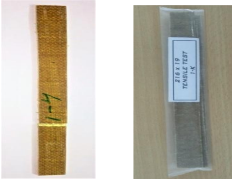
Fig 1. Tensile specimens before and after the test of jute kevlar epoxy composite
