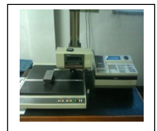
Fig. 2. Surface roughness measurement
