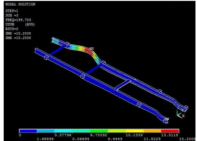
Figure 5: Third mode of vibration with maximum deformation.
