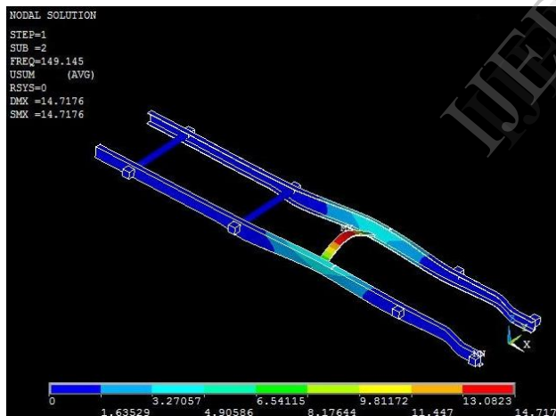
Figure 4: Second mode of vibration with maximum deformation
