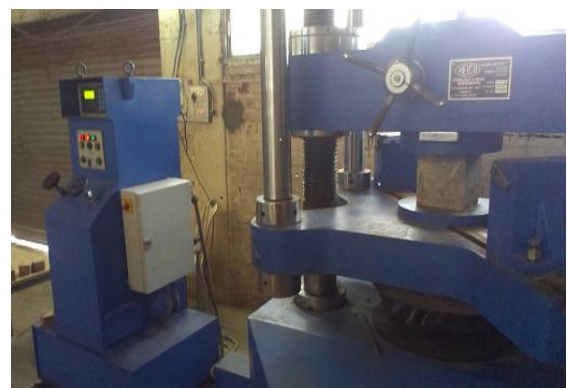
Fig 3. Testing of concrete cubes
