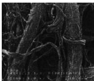
Fig. VIII Treated sample cause fibrillation
