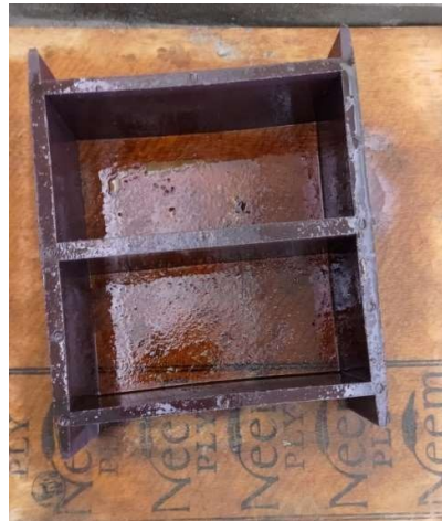
Figure 7: Wet mix mould
