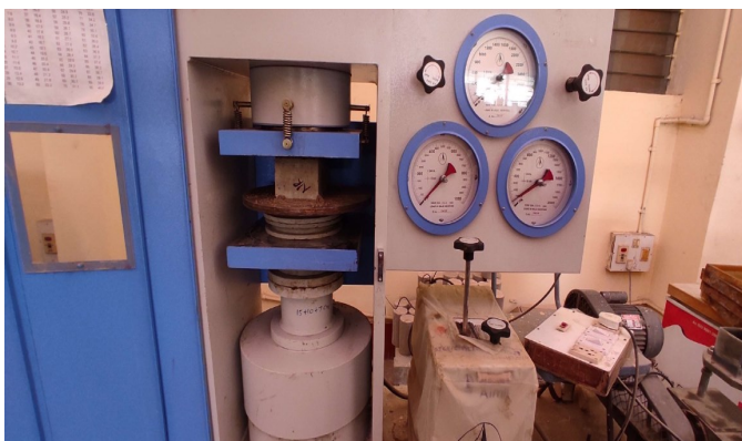
Figure 10: Set up of compression testing machine
