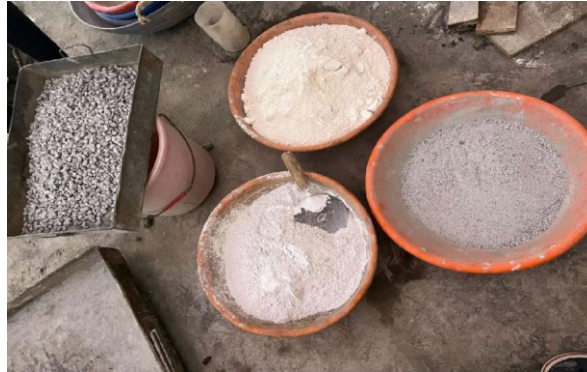
Figure 6: Materials which are weighed according to calculation
